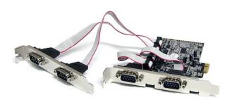
The PEX4S553 4-Port Native PCI Express RS232 Serial Adapter Card with 16550 UART lets you add 4 RS232 (DB9) serial ports, using a single PCI Express expansion slot.
